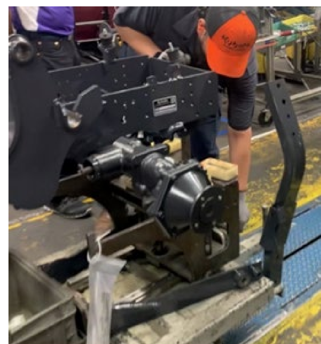
Figure Caption: An operator having to manually pull the cart and drop the pin to the conveyor chain
