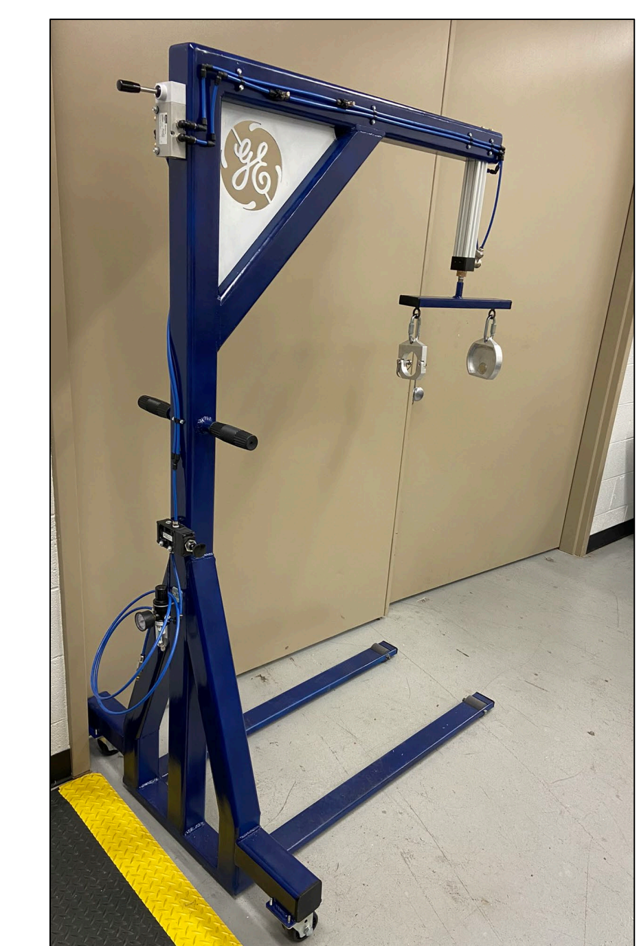
Figure 7.3. Rear view of hoist with pneumatic components
