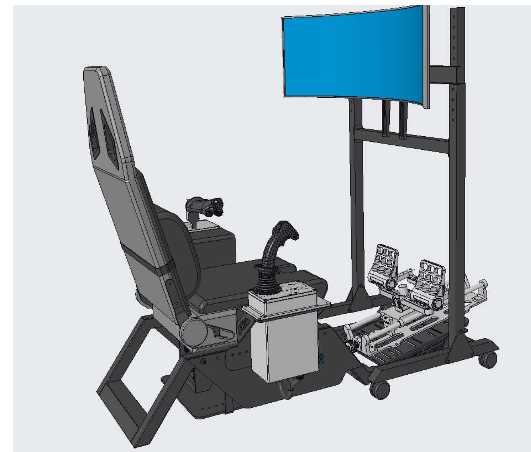
Flight Simulator Rig with Flight Stick, Throttle, Rudder Pedals, and Gaming Monitor
