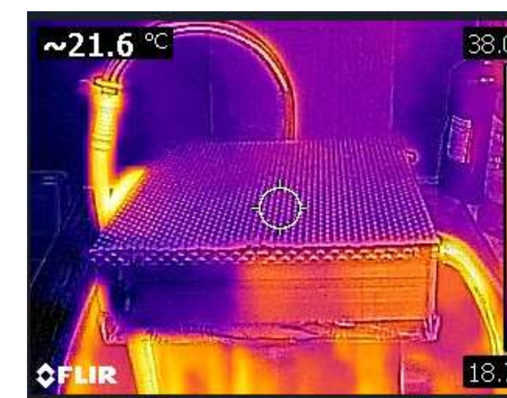
Early testing using spray foam for insulation (no heat compound or aluminum-wrapped PEX)
