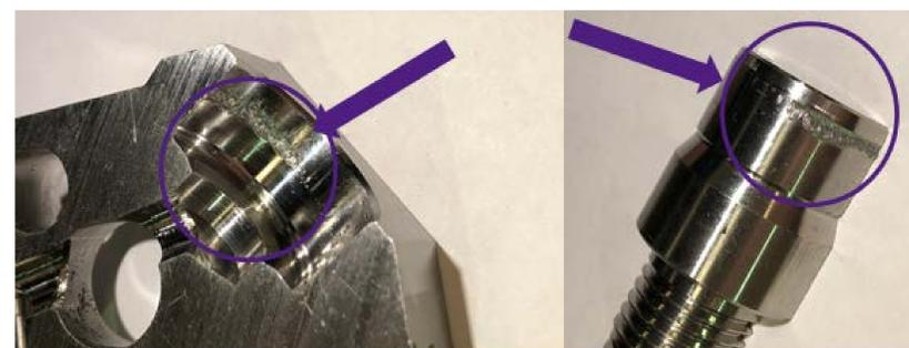
Upon receiving part samples from Stanadyne that had been cut by a diamond saw, galling was visually evident on both mating surfaces. The photographs to the left illustrate the galling on both the housing and valve.
