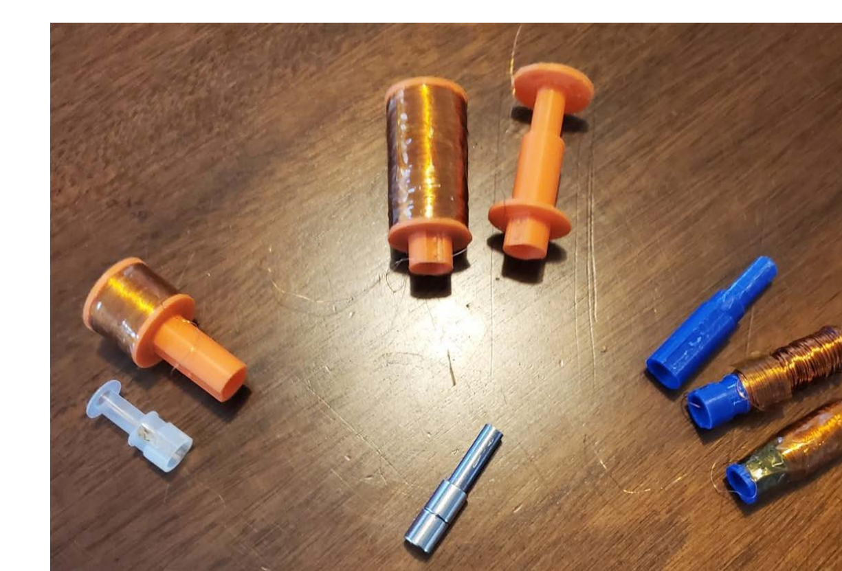
Fig. 7 Various printed bobbins. Far left: original bobbin. Top Centered; printed versions of Figs. 1+2.
