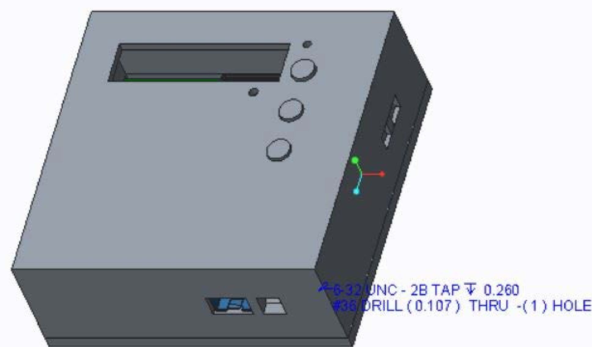
Above: Final case design assembled in Creo with button and slide switch actuators and a 3D model of this year's board
