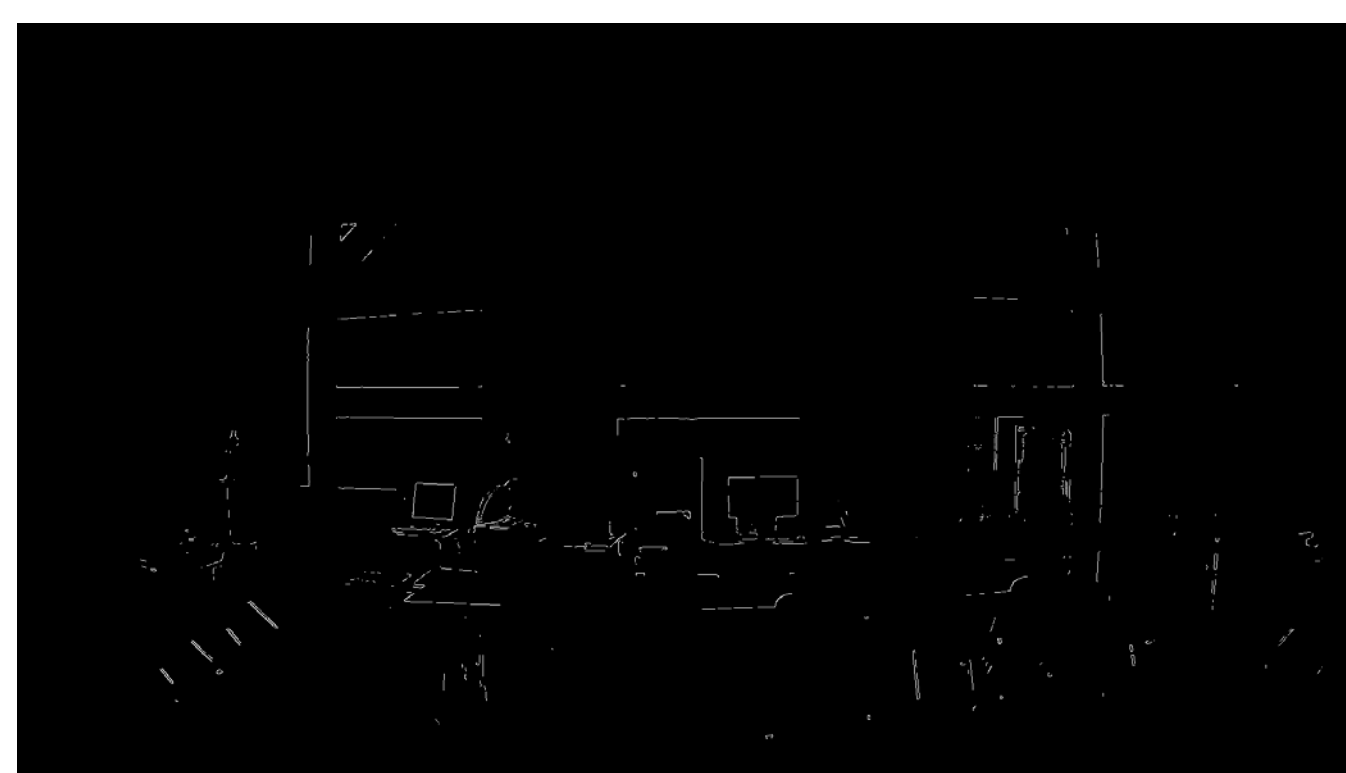
This is the above photo of the room filter. Each of the white lines are contours, which is what was used to identify the crew members. There is a lot of contours that can be seen, which makes for a lot of data that is going to throw the readings off.
