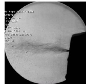
Figure 4: Mist From Compressed Body Spray (Shadowgraph Imaging)
