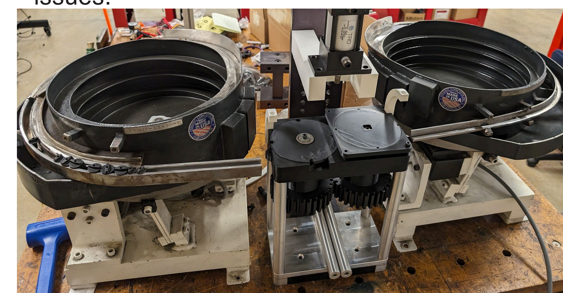
An overhead view of the team's deliverable, with the selector knob feeder bowl on the left, and the zerk fitting feeder bowl on the right, converging towards the pressing mechanism at the center.
