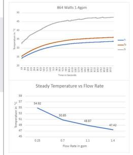
To further explore performance the rig was "stress tested" from no-load (0 Watts) and room temperature to the maximal achievable load (864 W). No heat shock was evident, and temperatures remained moderate.
