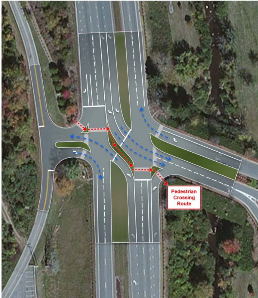
Figure 20 - RCUTS Intersection Concept at Centennial Drive Entrance
