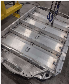
Complete battery tray, part that is being inspected
