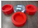
Concept 1 disposable PLA cups to fix samples to using UV curing resin
