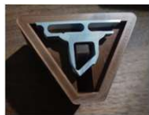
Sample clamp proof of concept bottom view with 140-120 sample
