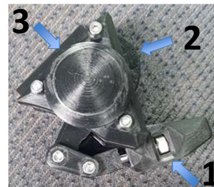
Assembled Sample Clamp 1 : The image shows the assembled clamp with the adjustable feature and finger guards. The interchangeable grips is also present. This allows comfort no matter the size of the hand.
